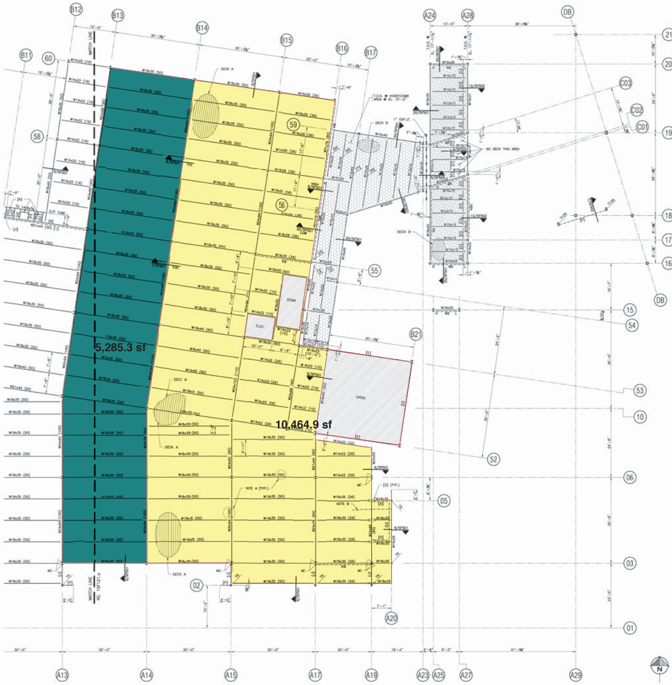
1 SECOND FLOOR FRAMING PLAN AND LOW ROOF FRAMING 1/8" = 1'-0" (T.O.S. @ EL. 18'-10 1/2" - U.N.O.)
